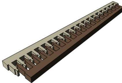
**Figure 7 Comb Drives Designed in AutoCAD and Exported to Carrara.**
