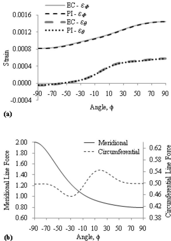
Fig. 5: Isotropic, variable thickness toroid (a) planar strains;
