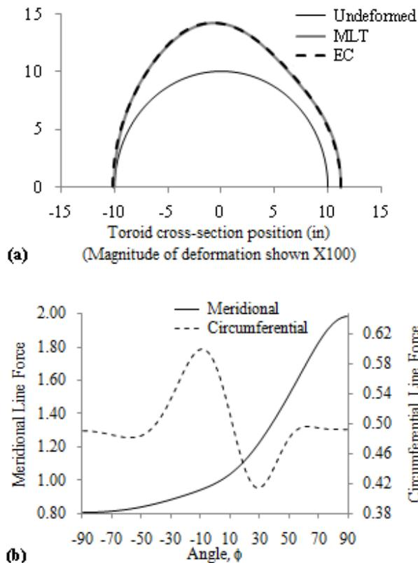
Fig. 4: Isotropic, constant thickness toroid (a) toroid displacement comparison; (b) FEA normalized line forces (EC and PI results identical)
