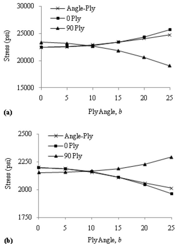
Fig. 9: Maximum layer stresses with respect to angle ply orientation
