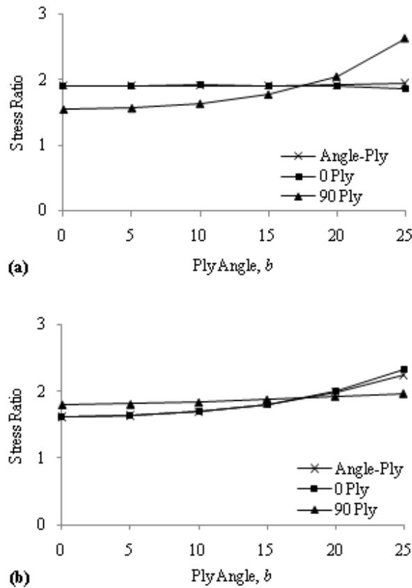
Fig. 10: Ratio of maximum to minimum layer stresses with respect to angle-ply orientation
