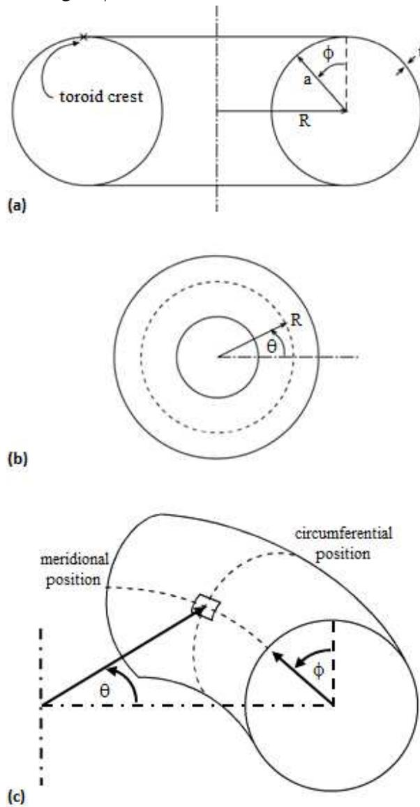
Fig. 1: Circular toroid geometry (a) section view; (b) top view; (c) global view
