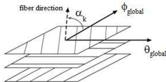
Fig. 3: Laminate fiber orientations
