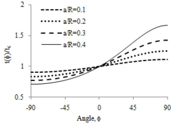
Fig. 2: Thickness variation with meridional position (normalized with respect to crest thickness,  $t_c$ )
